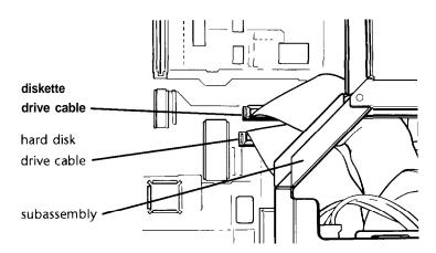
Grasp the connector and pull it straight up to remove it from the socket. Do not pull only on the cable.
